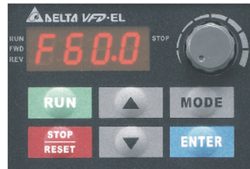
Figure 2: VFD control panel
