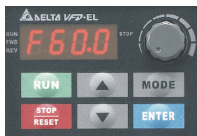
Figure 6: VFD control panel
