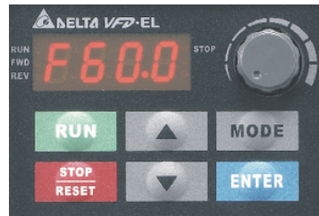
Figure 3: VFD control panel
