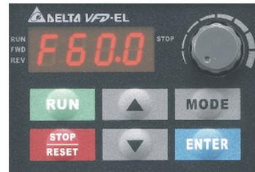
Figure 8: VFD control panel
